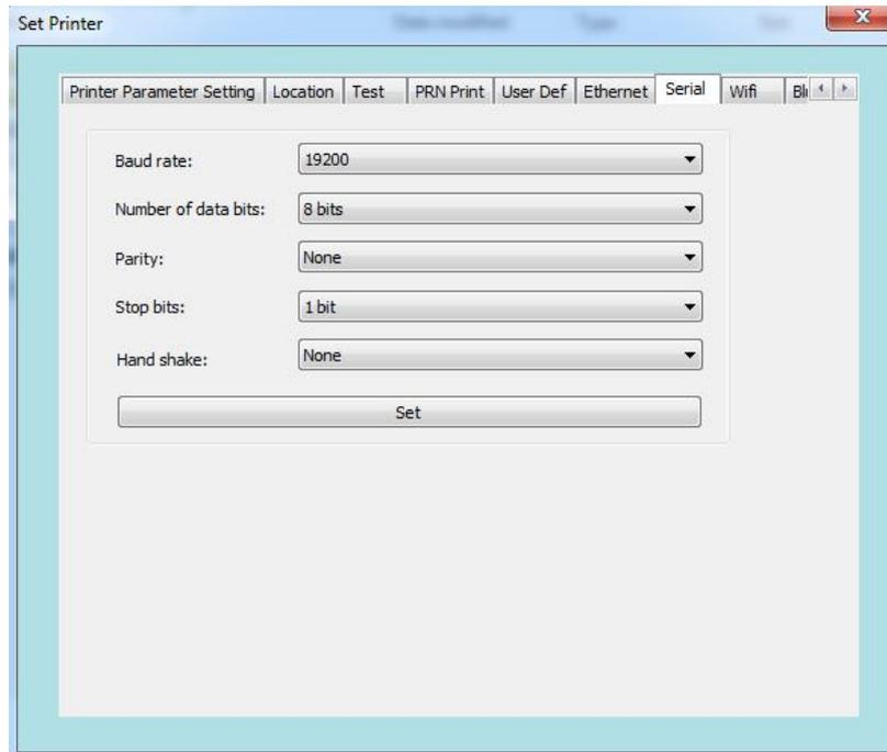
Switch to serial port setting interface to set serial port parameters. interface to set serial port parameters.
