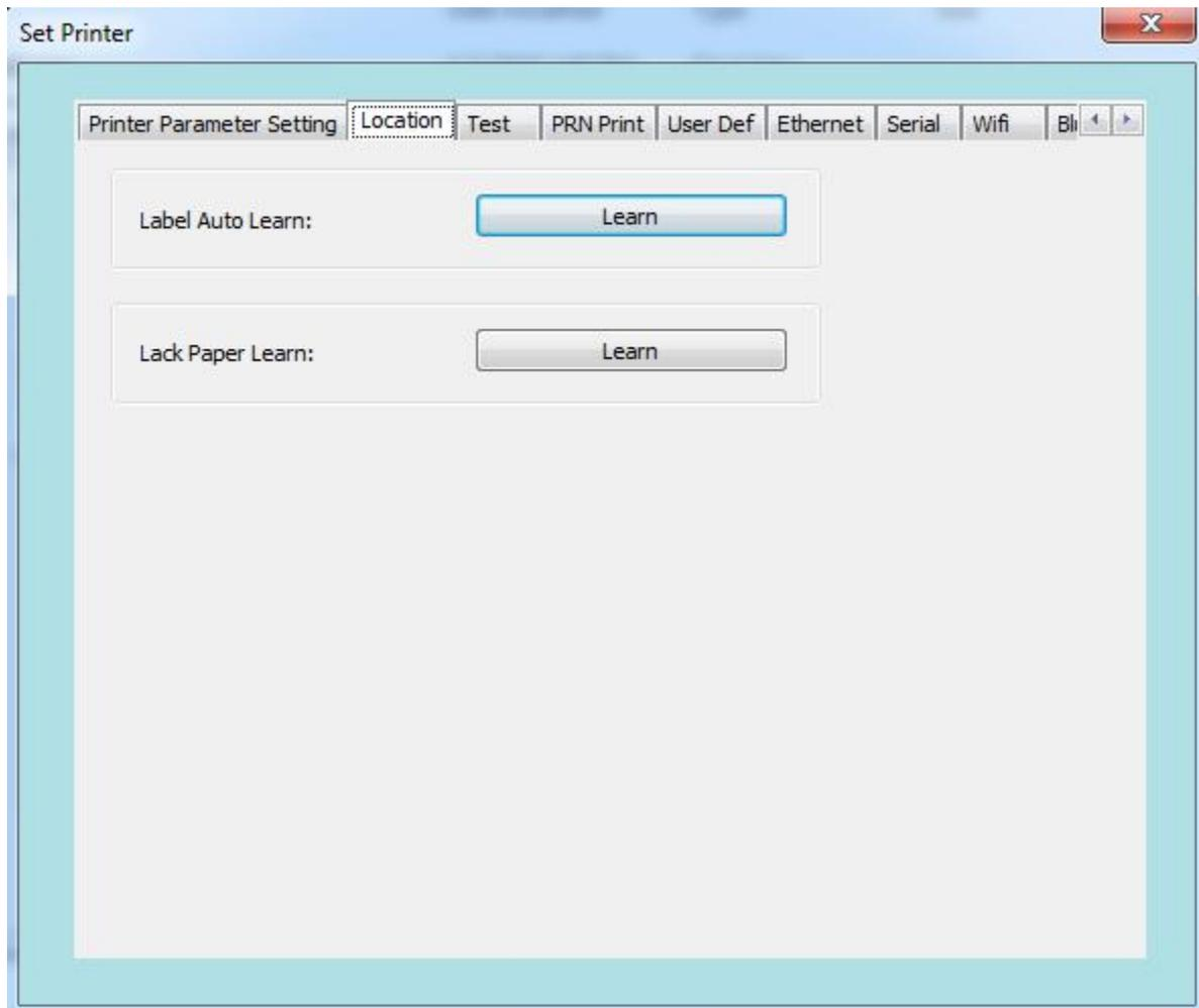
When the printer is ready, switch to the label calibration screen.
