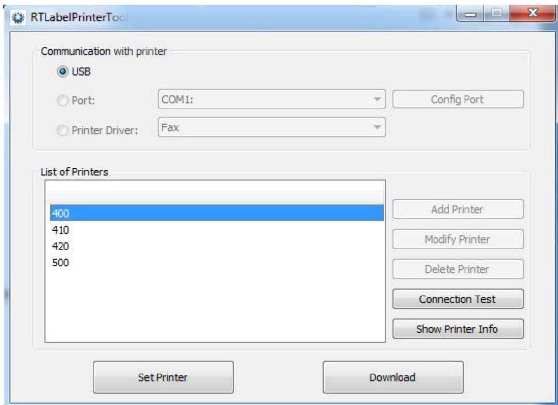
According to the model interface, select U or other port or driver port to connect the printer, and click [Connection Test]. If the following figure is displayed successfully, it means that the printer has been connected.
